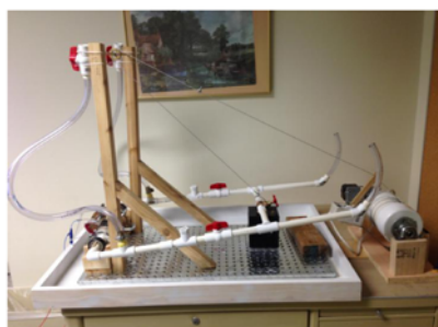
Figure Four. Actual model used in this study. The model was constructed of polyvinylchloride pipe, with gate valves in each limb to change resistance. Using two polycarbonate cups that mated together through a manufactured pressure plate, and the membrane was sandwiched between the pressure plates. The fibrillar transducer-tipped catheters were inserted into the polycarbonate cups. The entire system was filled with water, with an open gate valve on the upper crosspiece, and the ends of the tubes were open to atmosphere. The polyvinylchloride piping was rotated by a motor, with the axis of rotation about the low transverse member containing the compliant membrane.
